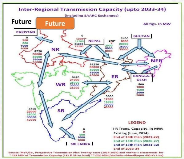
Significant Transmission System Interconnection (Both AC and DC) are being Planned and Proposed.
